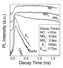
Fig.2. PL decay curves of the x=0.1% sample monitored at GaAs PL, E<sub>b</sub>, NN<sub>E</sub>, NN<sub>D</sub>, and NC.
