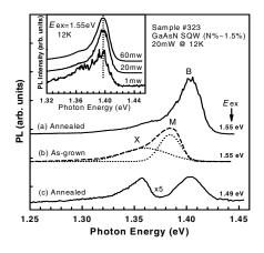
Fig.5. Comparison of the low-temperature PL spectra of the as-grown and annealed  $GaAs_{0.985}N_{0.015}/GaAs$  SQW under different excitation energies. The inset shows the 12 K PL spectra of the annealed sample under different excitation power.
