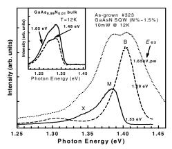
Fig.4. 12 K PL spectra of the  $GaAs_{0.985}N_{0.015}/GaAs$  SQW under different excitation energies. The inset shows the selectively excited PL of  $GaAs_{0.99}N_{0.01}$  bulk sample.
