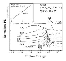
Fig.1. PL spectra of the GaAs<sub>1-x</sub>N<sub>x</sub> sample (x=0.1%) under cw excitation at various temperatures. The inset shows the integrated PL intensity as a function of excitation power.
