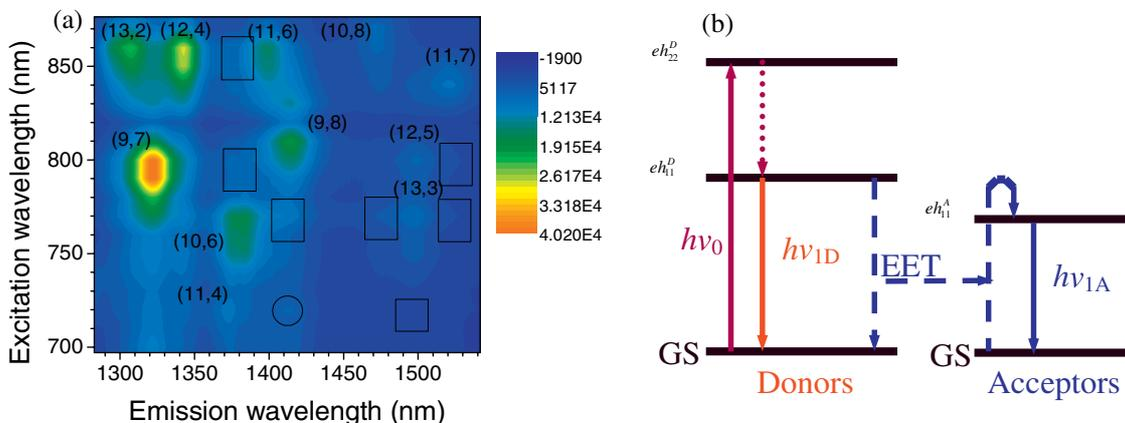
**Fig. 2** (online colour at: [www.pss-b.com](http://www.pss-b.com)) a) PLE map, showing exciton–exciton resonances and EET features (squares and circles); b) schematic mechanism of exciton relaxation in bundles [21].
