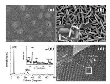
Fig. 1. (a) Low-magnification and (b) high-magnification SEM images of the nanoplates. The SEM image in the inset (b) was taken under a tilted scan angle. (c) Typical XRD pattern of the  $WS_2$  nanoplates, in which all the diffraction peaks can be assigned to pure 2 H (hexagonal)  $WS_2$ . (d) HRTEM of a single nanoplate.
