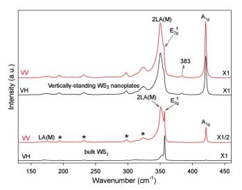
Fig. 2. Raman spectra of bulk  $WS_2$  and the present vertically standing  $WS_2$  nanoplates under VH and VV configurations, where VH (VV) means that the incident light is perpendicular (parallel) to the scattered light.
