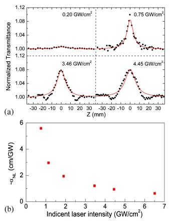
Fig. 3. (a) Open-aperture Z-scans of the WS $_2$  nanoplates on quartz substrate obtained under 25-ps, 532-nm laser excitation. The solid lines represent the best fits of the experimental data. (b) The measured nonlinear absorption coefficient ( $\alpha_{NL}$ ) values versus the incident laser intensity of the nanoplates.
